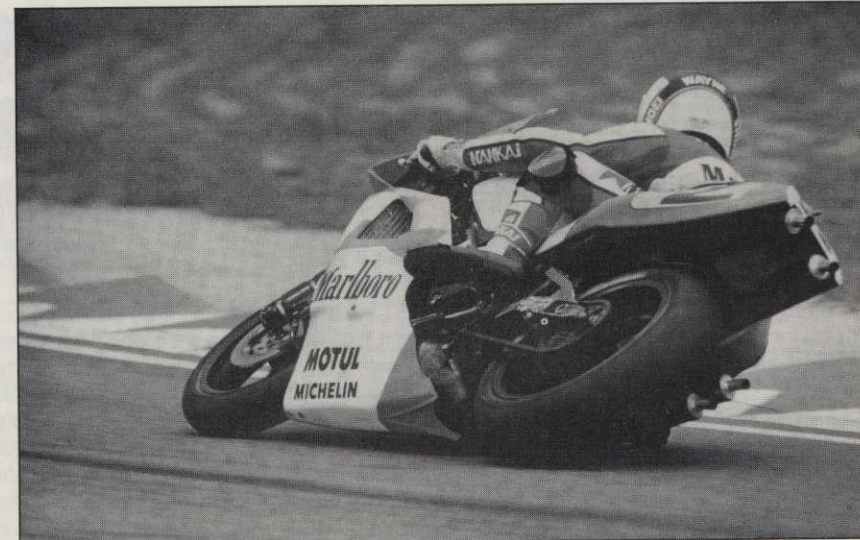
Defending 500cc World Champ Wayne Rainey says gearbox-ratio selection is among the most critical aspects of setup at Laguna Seca, affecting drive and handling characteristics.
